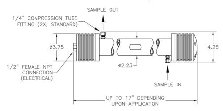
NOTE: ALL FLOW CELLS HAVE TWO 1/4"-20 X .30" DEEP MOUNTING HOLES LOCATED ON THE BACK SIDE
