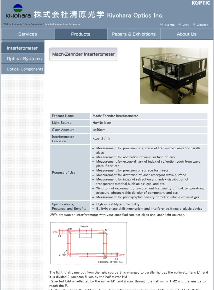
On the other hand, the light which was transmitted from the half mirror HM1 is reflected to both the mirror M2 and the half mirror HM2, and it runs through the lens L2 and reaches P.
