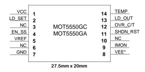
The laser output current can be modulated, if desired, through the input set pin, with a modulation small signal bandwidth in excess of 1MHz. The monitor output is also wide bandwidth allowing the modulated current to be monitored.
