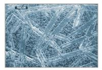
resulting in the formation of randomly oriented, interlocked, sheet-like fluorphlogopite mica crystals within the alumino-borosilicate glass matrix. The volume percent crystalline phase after heat treatment is approximately 55% with a mean crystal size of 20 microns. It is this uniform distribution of randomly oriented mica within the parent glass that gives rise to the unique characteristics of MACOR®.
