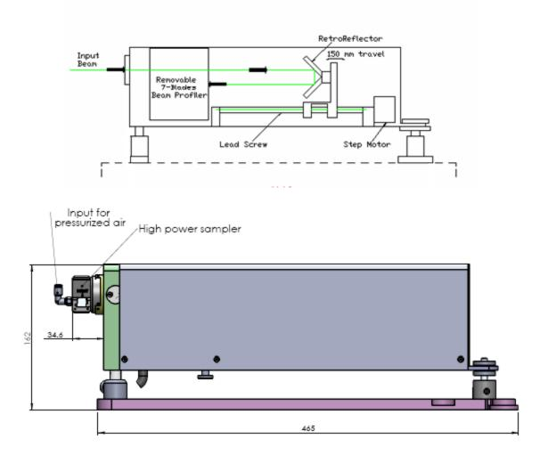
Mechanical configuration (optional SAM3-HP high power beam sampler)
