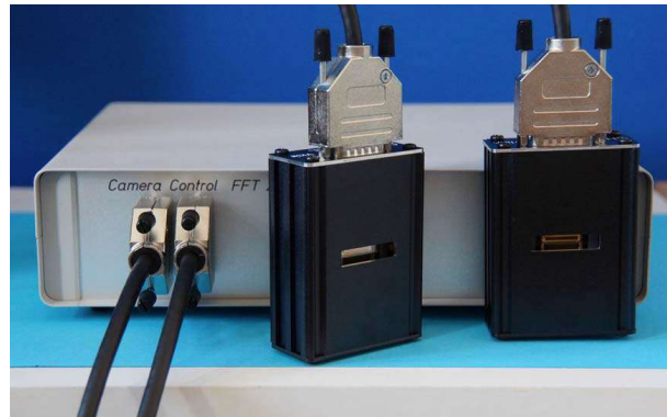
Camera Control with 2 sensor heads
