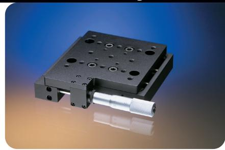
MacroMech 25 mm side driven linear stages are supplied with a high quality micrometer which is clearly marked for 0.01 mm accuracy over the full 25 mm of travel (1/2 division is equal to 5 μm). The micrometer drive can be
