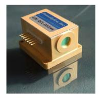
Model 1101-XX-CW-YYYY-BF is OEM version of Pranalytica's high power, continuous wave, room temperature midwave infrared laser system. It provides up to 3.5 W of continuous wave, room temperature (CW/RT) optical power at the wavelength of 4.6 µm or up to 2.5 W of CW/RT power at 4.0 µm. The butterfly package includes the high power quantum cascade laser mounted on a thermoelectric cooler, a thermistor to sense the QCL temperature and appropriate optics for collimating the output from the QCL.
