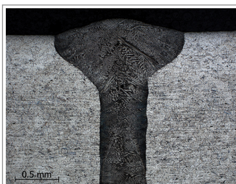
Keyhole laser welding - full penetration on 1/8" Inconel 800
