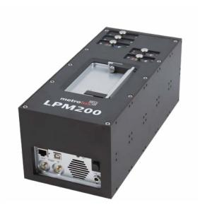
⇒ The Laser Propagation Monitor 200 (LPM200) is a beam profiler for automated determination of the focusing ability and beam quality parameter M² of lasers in industrial applications. Measuring M² and caustic only requires about 10 seconds.
