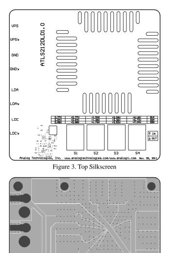
Figure 4. Top Layers without Top Screen Layer
