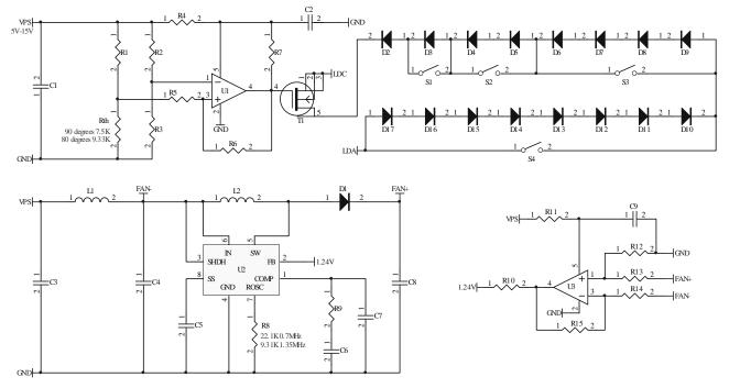
Figure 7. Schematic of ATLS212DLD1.0
