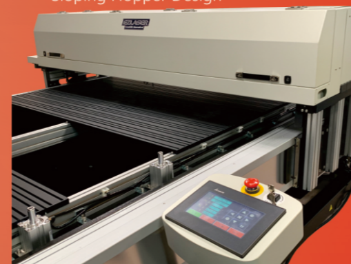
Standalone 7" LCD Color Touch Panel Cnornr Positioning Module (Option)
