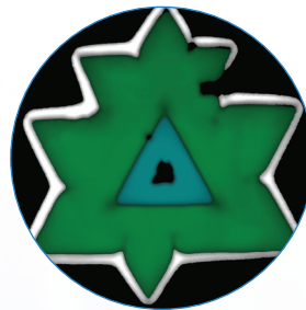
Ultra low frequency Raman and Photoluminescence image of a \text{WSe}_2 - \text{WSSe} - \text{WS}_2 heterojunction structure
