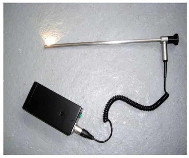
The Portascope Kit is an effective instrument to allow inspection and examination of normally inaccessible areas.
