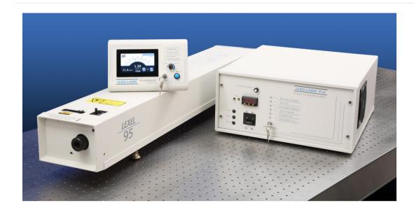
Our standard LEXEL™ PRISM Argon laser provides multiline output from 457nm to 528nm with output from 1W to 7W, plus tunable singleline wavelengths from 454nm to 528nm. With optional wavelength output in the mid-UV 351nm and 363nm or infrared at 1090nm. All user controls and system parameters are accessible via our new USB iController touchscreen remote using the latest 32bit ARM Cortex technology.
