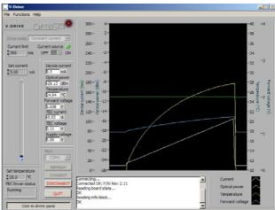
The LDR1500E laser driver module provides a versatile and user friendly platform for stable current and TEC control of Raman and 980nm pump lasers etc. The fully integrated digital Eurocard modules are designed for device characterisation, prototype development and experimental systems and offer easy device integration, full PC control and monitoring, or set & forget operation utilising the on-board EPROM.
