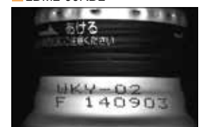
It is possible to illuminate the whole thing evenly to form an image of the text.
