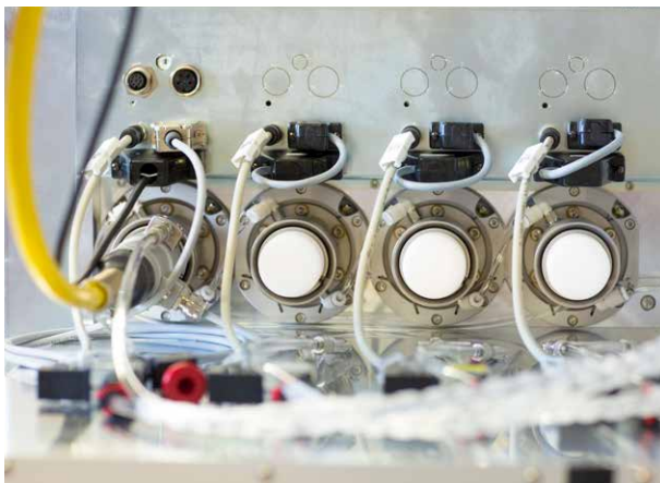
4-exit beam switch
