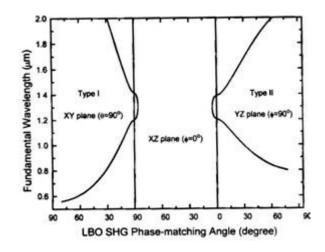
LBO is phase matchable for the SHG and THG of Nd:YAG and Nd:YLF lasers, using either type I or type II interaction. For the SHG at room temperature, type I phase matching LBO can be reached and has the maximum effective SHG coefficient in the principal XY and XZ planes in a wide wavelength range from 551nm to about 2600nm. LBO optimum type II phase matching falls in principal YZ and XZ planes.
