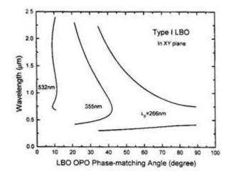
LBO is an excellent NLO crystal for OPOs and OPAs with a widely tunable wavelength range and high powers. LBO OPO and OPA that are pumped by the SHG and THG of Nd:YAG laser and XeCl excimer laser at 308nm have been reported. The unique properties of type I and type II phase matching as well as the NCPM leave a big room in the research and applications of LBO's OPO and OPA.
