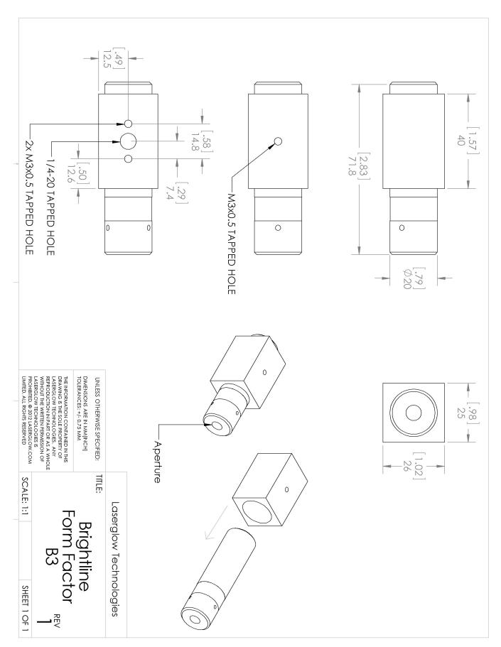
Product Datasheet generated on 2015-08-08 for Part Number: BOP005259 - LBD-660 Brightline Pro Complex Pattern Projecting Laser - Page 4 of 6 Laserglow Technologies - 416-729-7976 - sales@laserglow.com Copyright 2015 Laserglow Technologies - All Rights Reserved
