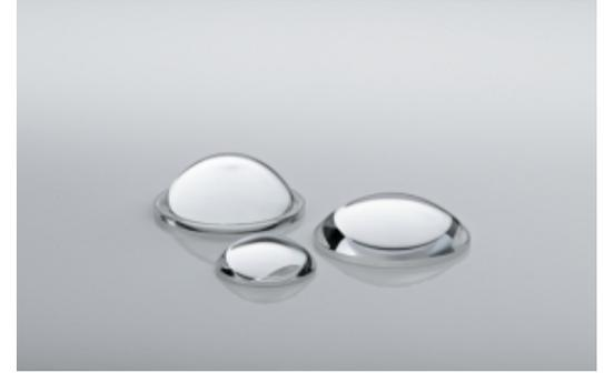
The non-spherical surface of an aspheric lens allows a single component to effectively focus or collimate even highly divergent emissions, potentially replacing a multi-lens system with a single aspheric lens.
