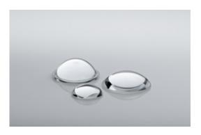
The non-spherical surface of an aspheric lens allows a single component to effectively focus or collimate even highly divergent emissions, potentially replacing a multi-lens system with a single aspheric lens.
