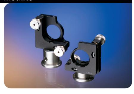
These mounts can be bottom mounted on a Half-inch Post, StablePillar™ or one of two riser blocks. Alternatively, they can be side mounted on a rod system carrier. Mirrors are retained in the mount by two delrin inserts and a nylon tipped set screw.
