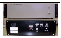
The laser energy is delivered out of a detachable optical fiber with a 0.6 mm diameter and 0.37 Numerical Aperture that attaches to the back of the unit. The unit incorporates an internal microprocessor that regulates the internal operations, and is controlled via a RS232 interface by an external computer.
