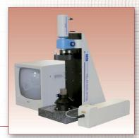
Vertical set-up for testing of flat and spherical surfaces and radius measurement.
