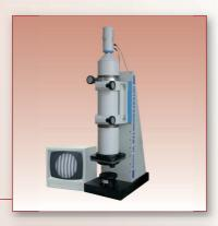
Vertical set-up for testing of flat surfaces with phase shifting.
