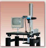
Workstation for quick testing of small plane optical components.
