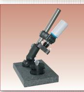
Inverted set-up for testing of flat and spherical surfaces as well as radii.
