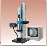
Workstation for testing of prism surfaces.
