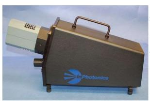
The "InPhochelle" is a compact Raman instrument offering high resolution (down to 2 cm-1) across the full spectral range (200-3500cm-1). The design uses fast f/2.8 optics for excellent throughput. Spectral acquisition is fast and highly reproducible. Since the only moving part is the shutter, the instrument is very rugged.
