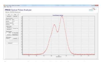
Spectrometer functionality displaying the second harmonic spectrum
