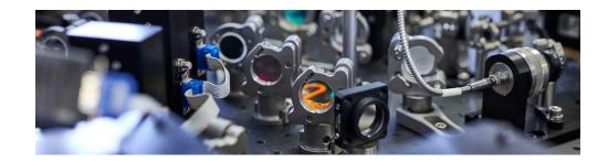
Your INFINITY microscope is assembled with standard optical and optomechanical components that are freely placed on a breadboard. This gives us 100% flexibility as we realize
