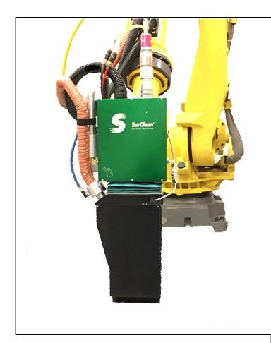
SurClean introduces the HyperDisc Laser Process Unit for high power laser ablation surface cleaning and preparation. This process head is lightweight but powerful and suitable for large area applications.
