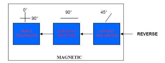
The reverse light by the output polarizer, through the faraday rotator under the magnetic field, rotating 45 degrees again in the same direction and becomes 90 degrees with the forward light, reflected or absorbed by the input polarizer.
