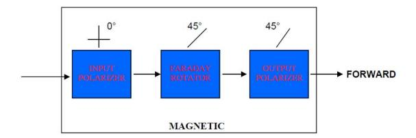
The forward light by the input polarizer, through the faraday rotator under the magnetic field, rotating 45 degrees and exits through the output polarizer.
