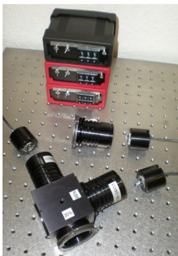
Two Wavelength Direct Fluorescence Configuration
