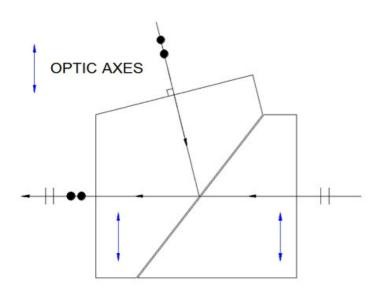
This special version of the Glan-Taylor polarizer is cut such that the rejected S-polarized light exits in a direction parallel to the side exit face normal. More importantly, if the beam
