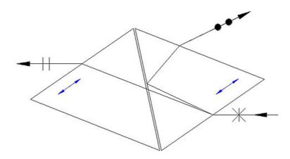
This special version of the Glan-Taylor polarizer is cut such that the P-polarization (extraordinary ray) intersects all four optical faces at Brewster's angle, thus ensuring a minimal insertion loss over a wide operating wavelength range. Transmission in fact is approaching 99% for the P-polarization and extinction ratio is exceptional, exceeding that of the more conventional cut Glan-Taylor.
