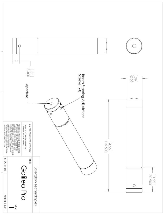
Product Datasheet generated on 2015-08-12 for Part Number: GGE003XXX - Galileo Pro Portable Alignment Laser Module - Page 4 of 5
