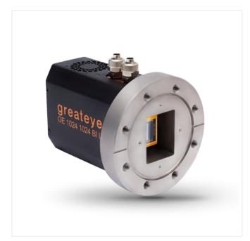
This series of highly sensitive, cooled cameras with vacuum flange is equipped with ultra-low noise 16bit readout electronics and perfectly suited for spectroscopy and imaging applications in the VUV, EUV and X-ray range up to 20 keV. The CCD detectors deliver spectra and images with outstanding dynamic range. To find the best solution for your application, greateyes offers various flange types and sensor technologies with quantum efficiencies up to 98%.
