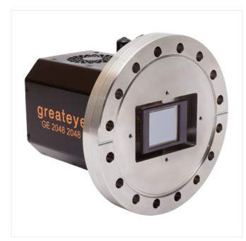
This series of highly sensitive, cooled cameras with vacuum flange is equipped with ultra-low noise 16bit readout electronics and perfectly suited for spectroscopy and imaging applications in the VUV, EUV and X-ray range up to 20 keV. The CCD detectors deliver spectra and images with outstanding dynamic range. To find the best solution for your application, greateyes offers various flange types and sensors with quantum efficiencies up to 97%.
