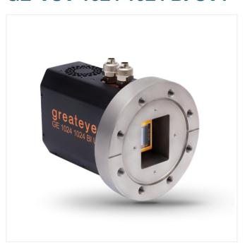
This series of highly sensitive, cooled cameras with vacuum flange is equipped with ultra-low noise 16-bit readout electronics and perfectly suited for spectroscopy and imaging applications in the VUV, EUV and X-ray range up to 20 keV. The CCD detectors deliver spectra and images with outstanding dynamic range. To find the best solution for your application, greateyes offers various flange types and sensor technologies with quantum efficiencies up to 98%.
