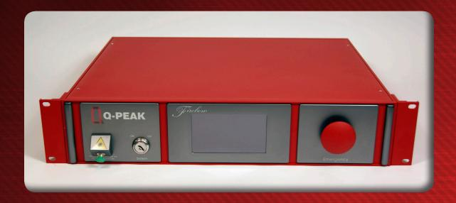
Q-Peak's Firebow CW 10-500 laser is a Tm:fiber based, compact, air-cooled unit containing resonator components, a pump diode, a diode driver, and a temperature controller in a single enclosure. The output fiber is endcapped and has a FC/APC connector. The system design allows for power scaling up to 500 W with non-connectorized pigtail fiber output.
