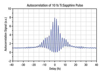
This interferometric autocorrelation was obtained using the OCTAVIUS-85M-HP. Precompensating mirrors were used to chirp the beam prior to the autocorrelator.
