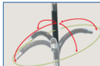
4 way articulation guides the viewer around corners and through dark recesses.
