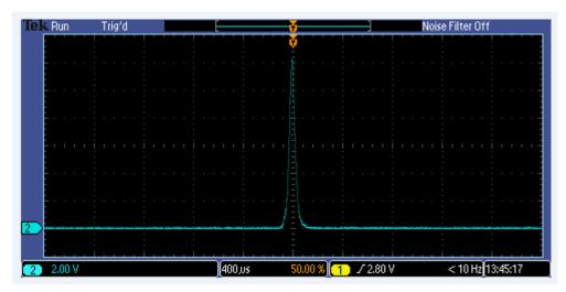
Commercial fiber laser (1552nm) pulse of 500fs duration.
