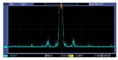
A weak satellite pulse, separated from the main pulse by ~ 7 ps appears when the AC trace is expanded vertically.
