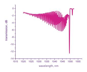
outside the fiber cladding. TFBGs are useful in sensing applications. Possible value of tilt angle is  $1^{\circ} \div 45^{\circ}$ . The TFBG transmission spectrum of 10mm length with tilt angle of  $3^{\circ}$  is presented in the graph.
