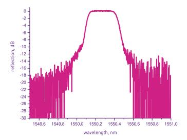
parameters (strength, FWHM, SLSR). Apodized FBGs are useful in sensing applications, signal and Brillouin scatter filtering and others. Possible value of SLSR for different grating strength is -10dB to - 30dB. The reflection spectrum of Apodized HR FBGs is presented in the graph.
