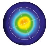
The standard FM100 is designed for all common YAG or excimer laser wavelengths, the model defines the precise optimization wavelength range and magnification of the system. In addition to the optional optimization of the contained optics for other wavelengths there are FM100 models for UV and even LWIR applications. The FM100LWIR-9600 for instance covers the Wavelength range from 9300 to 9600 nm for the measurement of CO2 laser foci.
