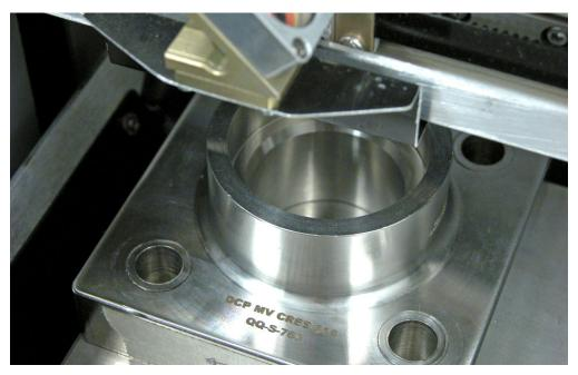
Non-Contact Marking: No Bits to Replace
