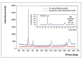
Reflections are in the desired range for these materials when using a Mn tube
