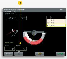
2. The graphics shows the detector direction. Markings on the circle shows active measurement point. Measurement value, and angular position for the detector (A).
