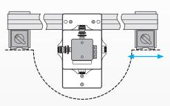
The setup of the bracket is very quick thanks to easily adjusted magnet bases and laser transmitter.
