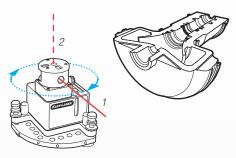
Option 1: the laser beam is used for a 360° sweep. Option 2: the laser beam is angled at 90° to the sweep.
