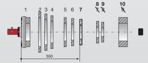
It's easy to add measurement points anywhere on the object in an existing measurement. The following points will be renumbered automatically. If you remove a point the following will be renumbered according to the same principle. If you remeasure a point, the old values will be saved in a history data base for possible later comparison. All this you can do at any time during the measurement!
