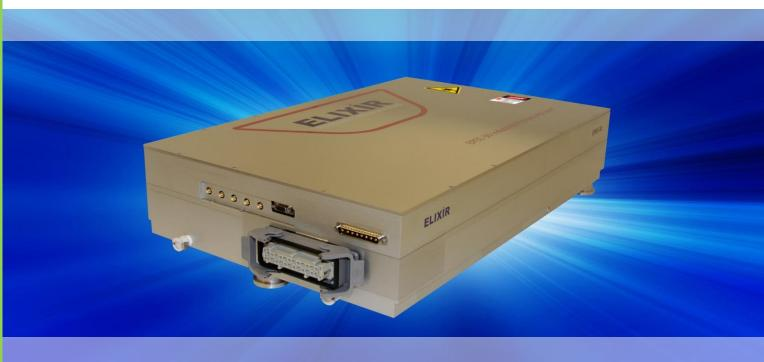
**EPEE-G15** combines advantages of fiber laser and free-space solid state amplifier technology and SHG technology to get >15 W output power with pulse energy over 100  $\mu$ J and pulse duration <15 ps at 532 nm wavelength.
