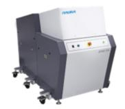
**EPEE 550 PECVD** is used in the manufacturing of LED chips and composite substrates. It is widely used in the deposition of SiO and SiNx dielectric films for LED blue-green and red-yellow devices and the high-speed deposition of SiO thick films on patterned sapphire substrates (PSS). In addition, the EPEE 550 PECVD tool supports high uniformity and low stress SiNx thin film deposition which can be applied to the development and mass production of third-generation semiconductor power devices.
