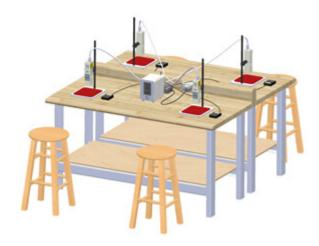
Users also have greater set up flexibility; for automated curing processes, the emitter can be mounted to robotic arms or further from the controller without fear of intensity variations. When used as a benchtop curing system, the unit can be paired with a stand and shielding for large area curing. It can also be used with multiple pathway lightguides for specialised applications when paired with MX spot emitters.
