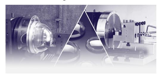
Our partner Phoenix Optical Technologies Ltd diamond turning facility operates 5 single-point machines to support our customers' growing demands for innovation and quality. This machining capacity is transformed into optical capability by a dedicated team of skilled technicians. We produce aspheric, free-form and diffractive surfaces in a variety of materials.
